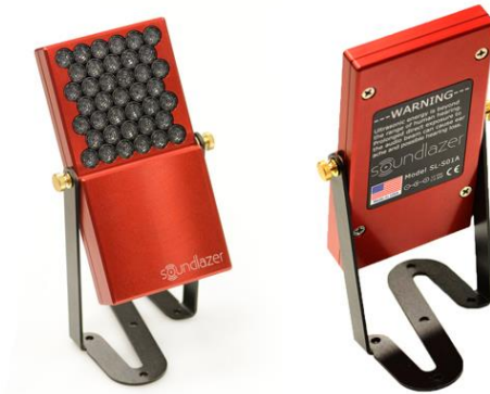
Figure 32: Soundlazer directional arrays
